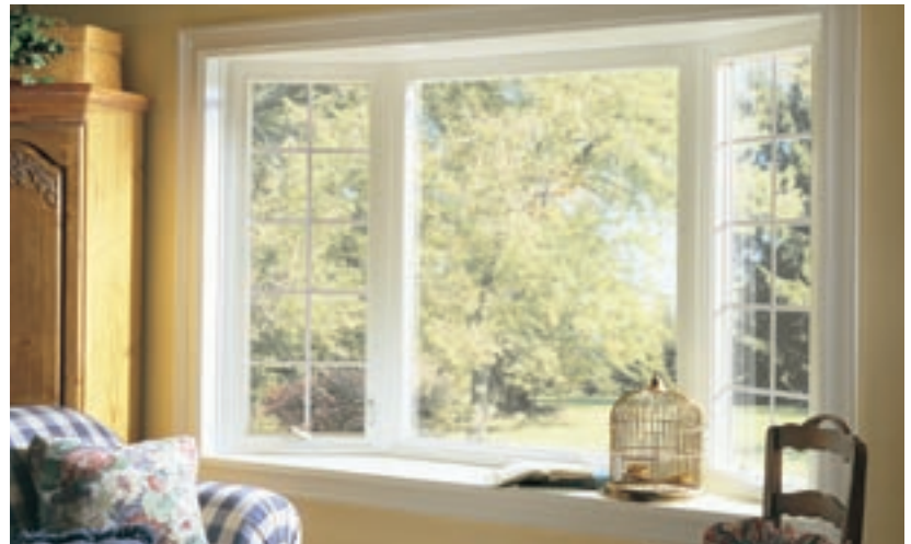
Bay windows , shown here with casement (sides) and fixed (center) windows, add architectural interest, plenty of light, and real spaciousness.
